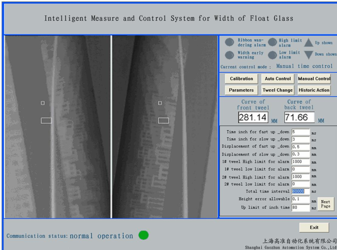
**Fig. 7 Interface of Parameter Setting**
